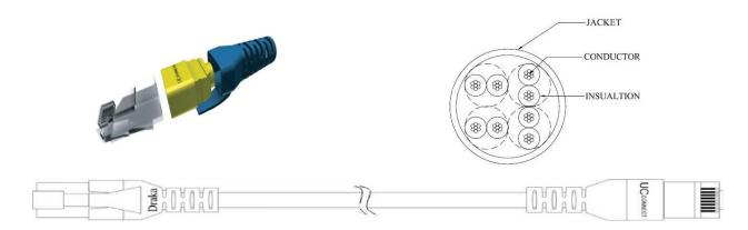
Stranded bare copper conductors insulated with thermoplastics polyolefin. Two insulated conductors twisted together to form a pair and four such pairs cabled to form the basic unit. Overall jacket with LSZH/PVC compound.
